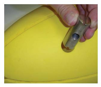
**Figure 5-4:** Crossbar Used to Secure Tail Cone Parts
