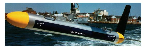
Figure D-11: Towfish with Standard Transducer Configuration
