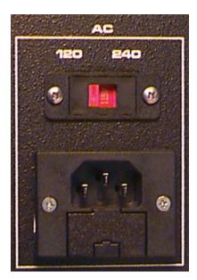
**Figure D-7:** AC Connector, Voltage Switch and Fuse on the Rear Panel of the TPU
