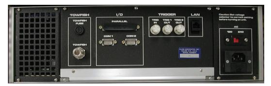
Figure D-6: TPU Rear Panel
