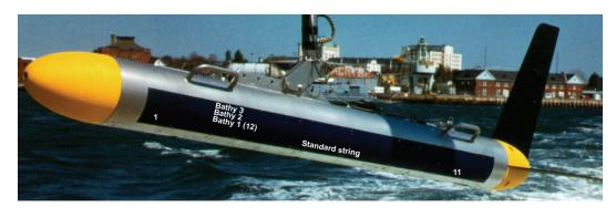
Figure D-12: Towfish with Bathymetry Transducer Configuration
