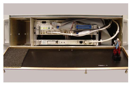
Figure 1-1: TPU—Shown With Access Panel Open
