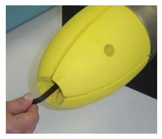
**Figure 5-2:** *Tail Cone being Aligned and Attached to Towfish*
