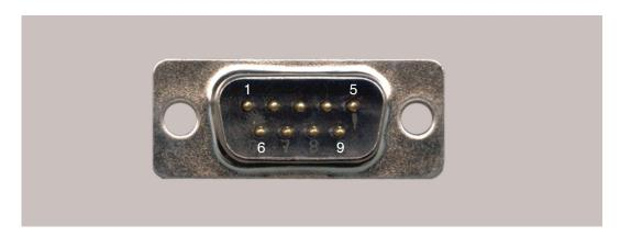
Figure 1-8: COM1 and COM2 Connectors
