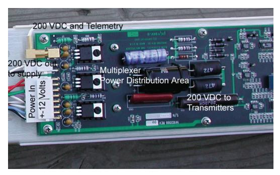
**Figure D-22:** *The Multiplexer Board*
